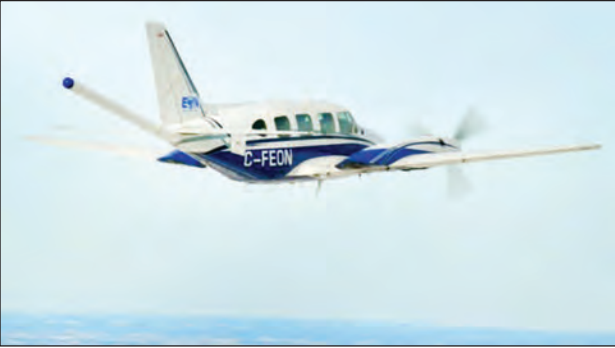
A Piper Navajo airplane with tail stinger magnetometer.
